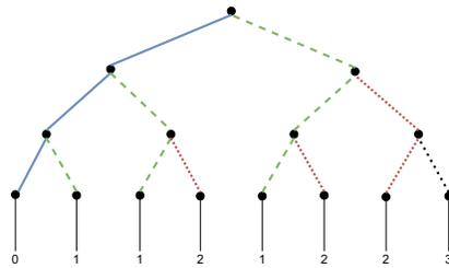
Fig. 2: Limited Discrepancy Search on a binary tree.
