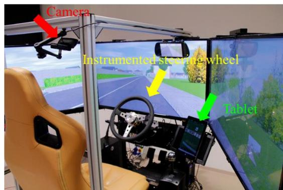
**Fig. 1.** The system set-up, with the steering wheel, the tablet and the camera
